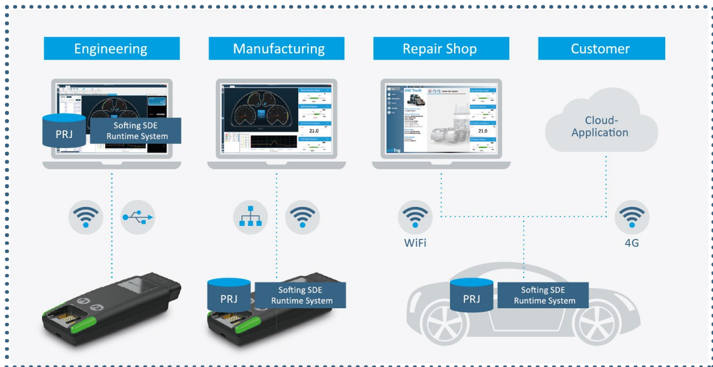
Fig. 2: Smart Architecture Enables Scaling
