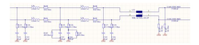
The following BR Filter is used in the old MediaConverter HW Version 2.0:
